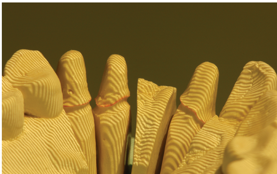
Fig. 1 White light projector pattern during the scanning process by an optical scanner
